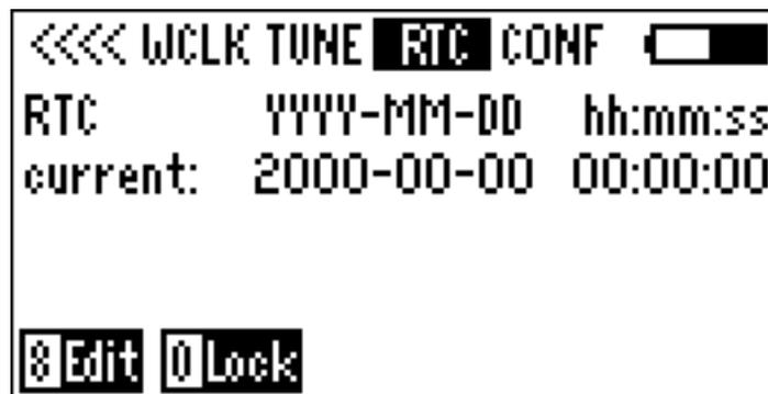
This menu sets the Real Time Clock. The RTC runs from its own battery and X-tal oscillator and contains all calendar data such as days in the month, leap year etc. It is an independent on board clock with its own battery and crystal. Note. **The RTC does not run from the tuned internal reference and is not as accurate.** It is used only to retrieve the actual time of day and the date when starting the time code generator and for logging purposes.
