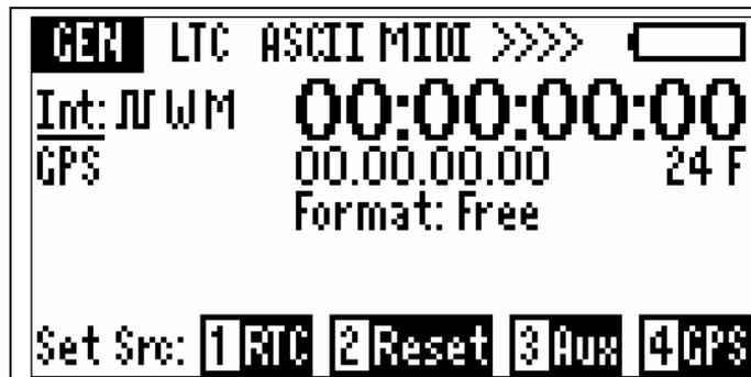
In this menu the time code generator parameters can be set. The generator starts from 00:00:00:00 and can be set from the following sources.
